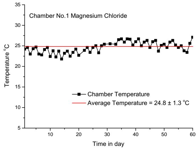
Figure 2.2: Temperature stability for chamber 1
