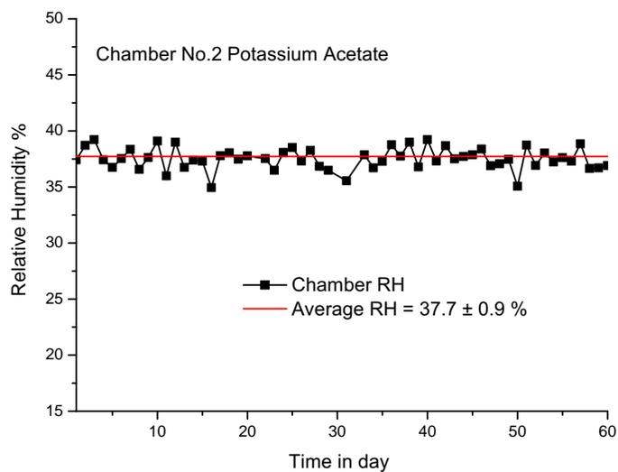
Figure 2.3: Relative humidity stability for chamber 2
