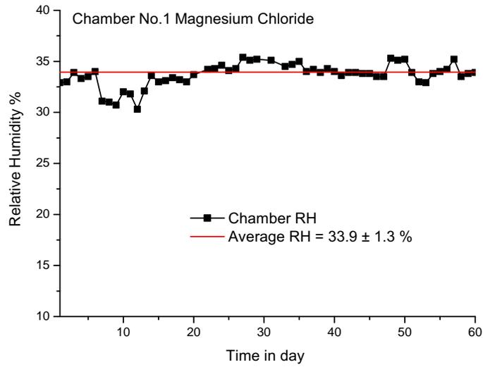
Figure 2.1: Relative humidity stability for chamber 1
