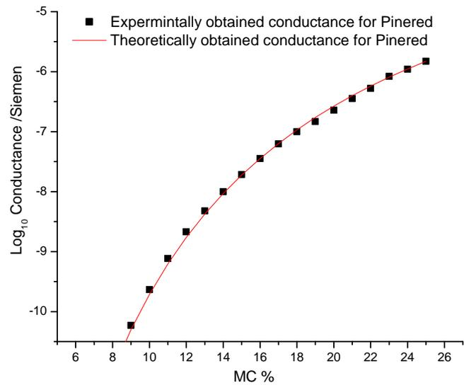
Figure 3.2: Log  $C$  vs MC for Pinered
