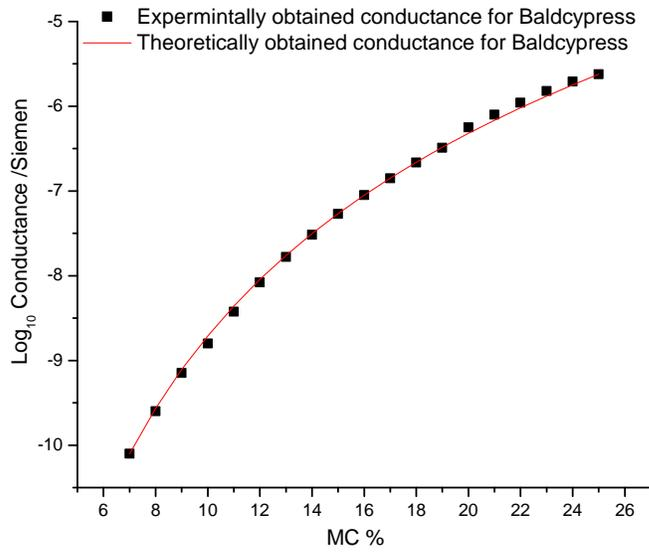
Figure 3.3: Log  $C$  vs MC for Bald cypress
