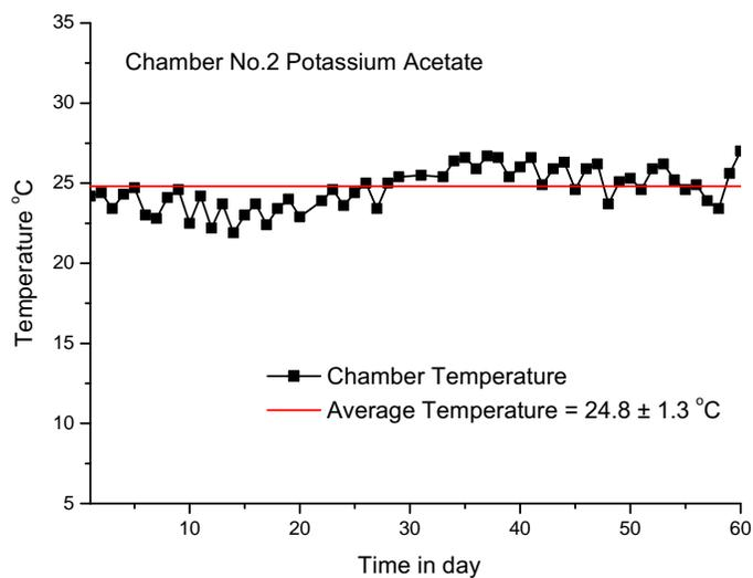
Figure 2.4: Temperature stability for chamber 2
